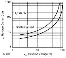
Figure 3. Reverse Current vs. Reverse Voltage
