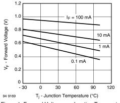
Figure 1. Forward Voltage vs. Junction Temperature
