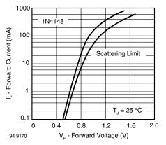
Figure 2. Forward Current vs. Forward Voltage
